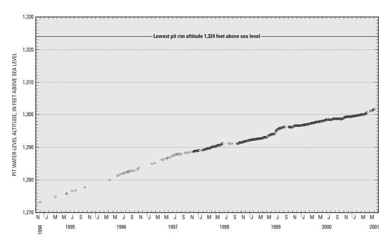
Figure 2. Water-level altitude in the Canisteo Mine Pit, Bovey, Minnesota, November 1994-June 2001.
