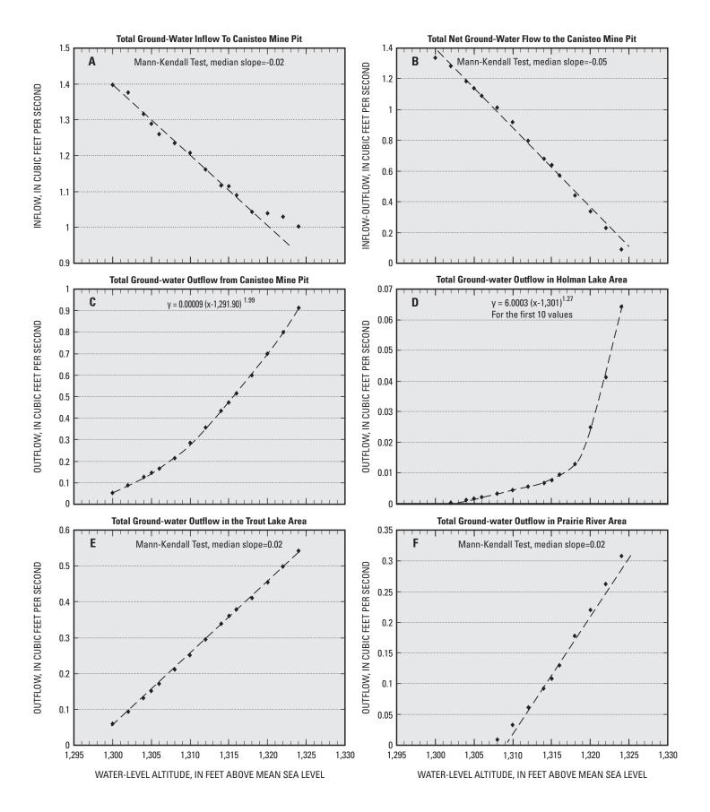
**Figure 9.** Simulated (A) total ground-water inflow, (B) total net ground-water inflow, outflow (C) total ground-water outflow rates from the entire pit, (D) ground-water outflow from the pit in the Holman Lake area, (E) the Trout Lake area, and (F) the Prairie River area at various constant pit-lake water-level altitudes for the Canisteo Mine Pit, Bovey, Minnesota.
