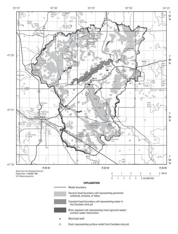
Figure 4. Model segmentation for MODFLOW simulation of aquifers surrounding the Canisteo Mine Pit, Bovey, Minnesota.
