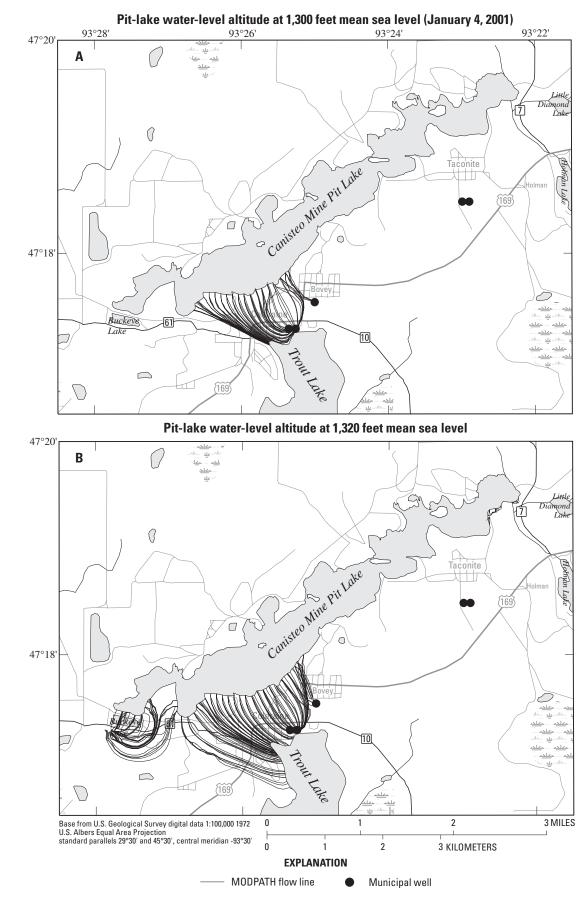
Figure 8. MODPATH flow lines for ground-water outflow from Canisteo Mine Pit at pit water-level altitude of: A.) 1,300 and B.) 1,320 feet above mean sea level, Bovey, Minnesota.
